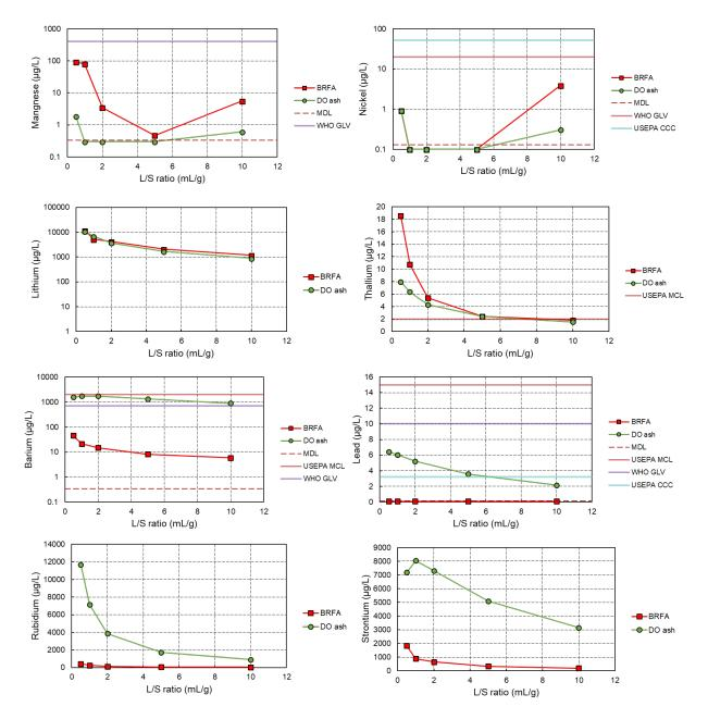
Figure 4. Concentrations (μg/L) of selected elements in the leachates over a range of liquid-to-solid (L/S) ratios under the LEAF Method 1316. MDL, U.S. EPA MCL, WHO GLV, and U.S. EPA CCC are plotted where available (Table 2).
