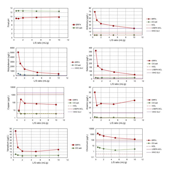
Figure 3. Final pH values and concentrations (µg/L) of selected elements in the leachates over a range of liquid-to-solid (L/S) ratios under the LEAF Method 1316. MDL, U.S. EPA MCL, WHO GLV, and U.S. EPA CCC are plotted where available (Table 1).
