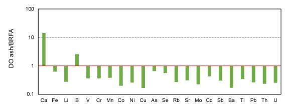
Figure 1. Comparison of bulk concentrations of trace elements in the DO coal ash sample with the U.S. fly ash sample.
