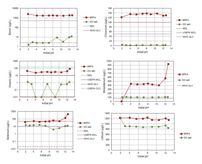
Figure 6. Concentrations (µg/L) of selected elements in the leachates over a range of initial leaching pH values under the LEAF Method 1313. MDL, U.S. EPA MCL, WHO GLV, and U.S. EPA CCC are plotted where available (Table 2).
