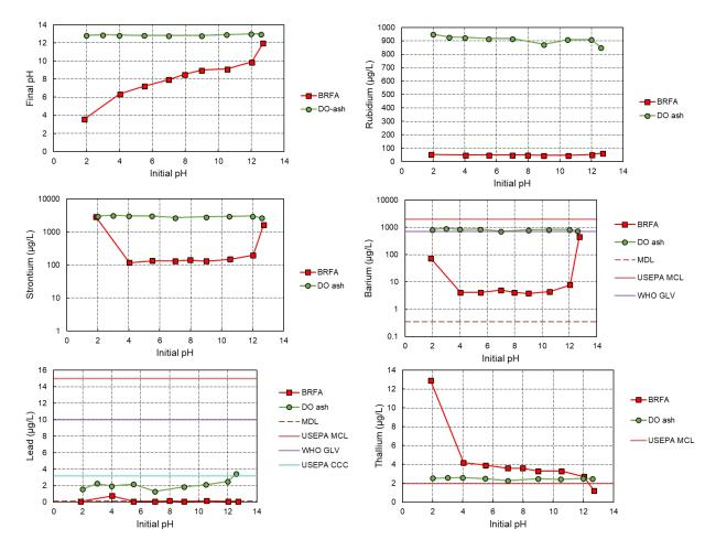
Figure 5. Final pH values and concentrations (μg/L) of selected elements in the leachates over a range of initial leaching pH values under the LEAF Method 1313. MDL, U.S. EPA MCL, WHO GLV, and U.S. EPA CCC are plotted where available (Table 2).
