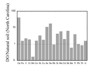
Figure 2. Comparison of bulk concentrations of trace elements in the DO coal ash sample with the average values of metals in North Carolina Soils.
