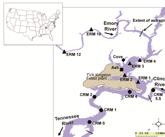
Figure 1. Map of the Kingston power plant site showing river sampling locations (rivers are in dark blue). Emory River sampling sites are marked using triangles ( \Delta ), Clinch River samples are marked using circles ( \circ ), and the cove samples are marked with a diamond ( \diamond ). Arrows below river names represent flow directions. Dashed lines indicate extent of ash found immediately after the spill.
